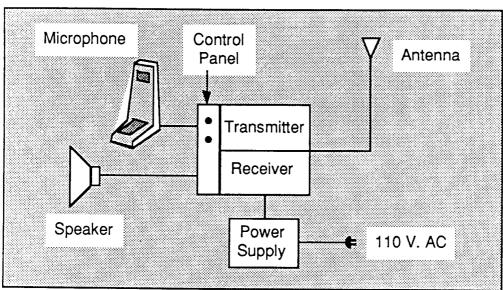
The base station contains a transmitter, receiver, power supply, and typically has a built-in speaker. The base station is usually powered by a standard 110-volt A.C. power source. A base station microphone and antenna are also required. In a simple system, the base station is merely a mobile unit mounted in a tray with a power supply for desktop use. The term "Control Station" is often used interchangeably with "Base Station."
