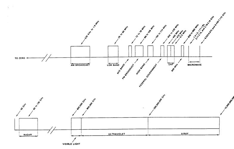
Although not technically accurate, the labels for each band in common usage today are shown in the chart below. Each of these specific bands have characteristics which offer advantages and disadvantages to radio users.
