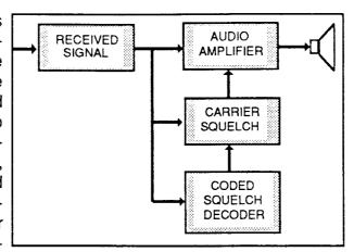
ines the demodulated squelch code and compares it to its own built-in preassigned code. If the codes match, the speaker opens up and the message is heard.
