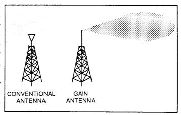
effective radiated power. This is done by channeling the antenna's radiation pattern in a particular direction and thus extending the distance it will cover. The use of a high gain antenna ensures better reception in the fringe areas of a system.
