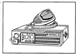
ately. Today, most mobile radios are compact enough to be mounted under, or near, the dash. These radios include a built-in speaker and have the controls located on the front panel.
