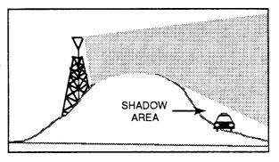
In the case where a hill causes a shadow, or hole, if we raise the antenna height, we can eliminate most of the hole. Thus, antenna height, to a large extent, cures terrain problems.
