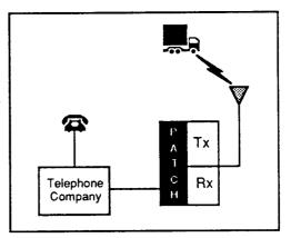
quest is then automatically interconnected to the telephone company and the call is completed over standard land line service.
