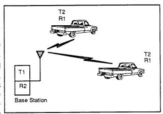
mobile transmits on frequency 2 and the base station receives on frequency 2. The mobile units cannot hear each other because their receivers are operating on a different frequency than their transmitters. The dispatcher is the only person who can hear all traffic.
