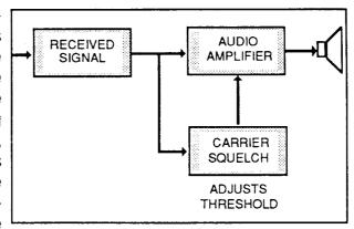
control is turned until the noise just stops. This position is called *threshold squelch*, and allows only the stronger message transmissions to be heard in the speaker. Other radios have a preset squelch level which is set to open at a predetermined signal strength.
