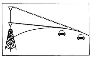
pends upon the effective height of the base station antenna. This is because other factors such as increased base station power do not increase range both ways. Basically the higher up in the air that an antenna can be installed, the greater an area that will be covered. This is because the radio waves follow a line-of-sight path.
