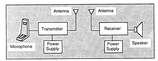
Located at the other end of this simple radio system is the receiver. Now the process is reversed and the receiving antenna picks up the radio signal and sends it to the receiver. Here the radio signal is processed into the original audio signal, which is fed into the speaker so that the original voice message can be heard.
