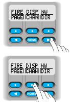
3. The display changes to show the zone name (on steady) and the current channel name (flashing). In the example shown, "FIRE" = Zone, "DISP NW" = Channel.
