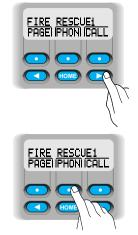
3. The display changes to show the last telephone number dialed or the last ID number transmitted/received. The **LIST** softkey also appears.
