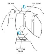
3. Press the bottom of the belt clip into the slot until it "clicks" into place. Pull outward on the bottom of the clip to ensure that it is secured to the radio.
