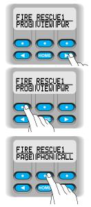
5. The display will show the first member in the list (name on the upper line, number on the lower line). The □ status indicator will appear (flashing), indicating you are in the programming mode.
