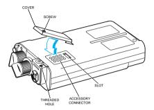
3. Snugly tighten the screw (0.3 in.-lb.) to hold the cover in place.
