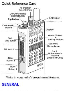
Turning the Radio On: Rotating the On/Off/ Volume Control Knob clockwise.
