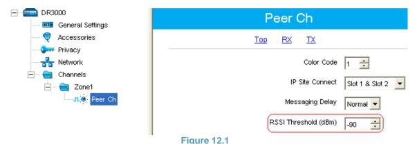
If the given repeater is able to operate on a dedicated RF channel (i.e. it is not required to share the channel with another system), then it's strongly recommended that the RSSI Threshold be increased from its default value of -115dBm to -90dBm. This will ensure that interference originating from a number of different sources does not prevent the repeater from transmitting.
