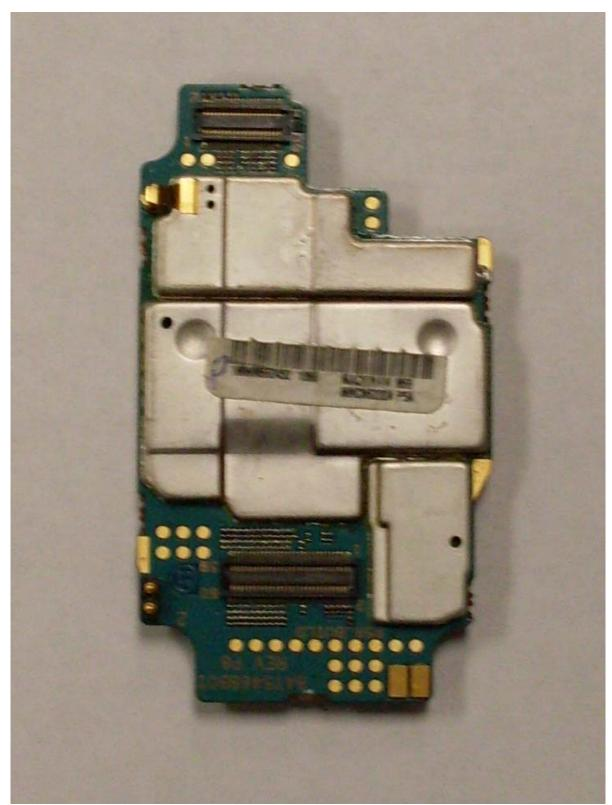
Vocon board with shields board (Bottom)
