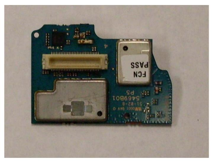
Expander board with shields board (Bottom)
