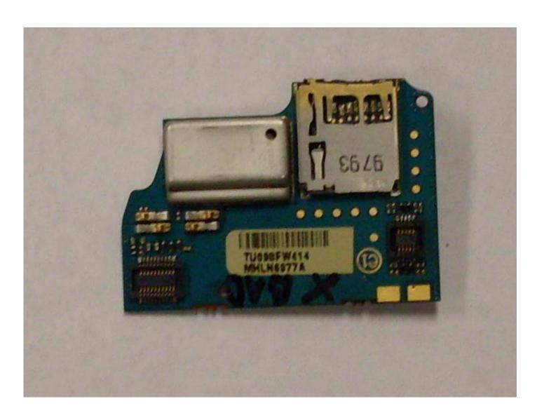
Expander board with shields board (Bottom)
