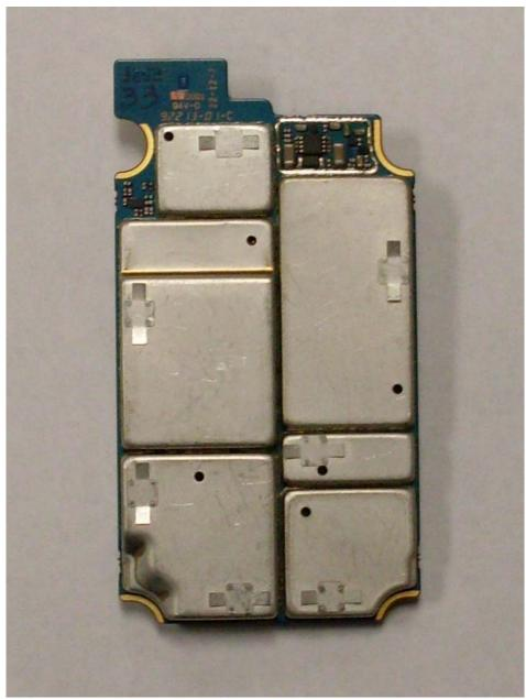
RF board with Shields (Bottom)
