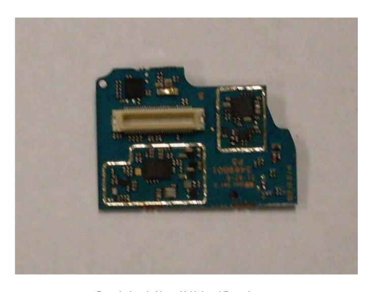
Expander board without shields board (Bottom)
