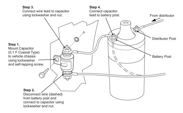
Figure 10-1. Ignition Coil Noise Suppression
