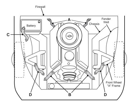
Figure 10-5. Ground Bonding
