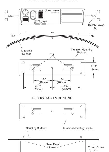
Figure 3-1. Transmission Hump Mounting (Top) and Below Dash Mounting (Bottom)
