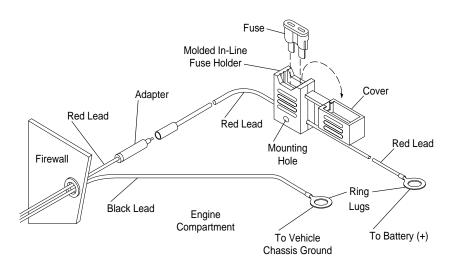
Figure 2-2. Power Cable Assembly
