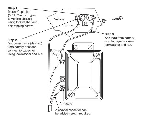
Figure 10-4. Voltage Regulator Noise Suppression
