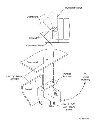
Figure 5-2. Mounting the Speaker Under the Dashboard
