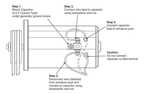
Figure 10-2. Generator Whine Suppression
