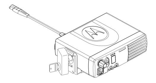
Figure 3-3. Locking Mounting Bracket (RLN4779)
