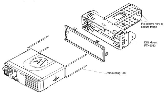
Figure 5-1. Fitting the Radio into the Frame
