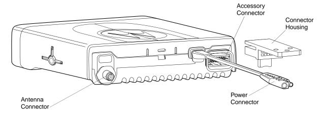
Figure 4-1. Connections to the Back of Radio
