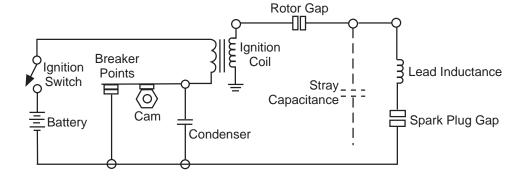
Figure 8-1. Typical Vehicular Ignition System, Simplified Schematic Diagram
