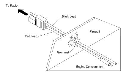
Figure 2-1. Power Cable Routing into the Engine Compartment
