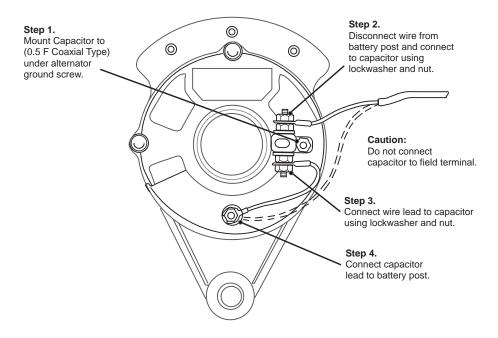
Figure 10-3. Alternator Whine Suppression
