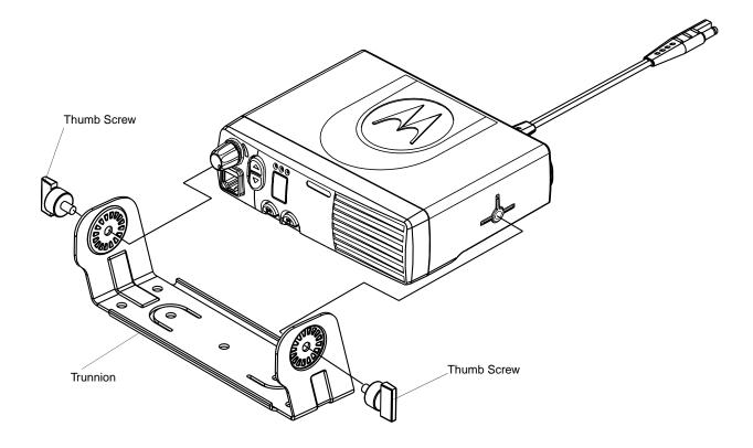
Figure 3-2. Radio into Trunnion
