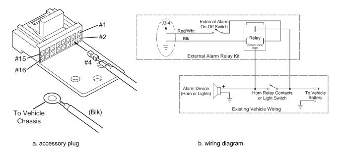
Figure 6-1. HLN9328 External Alarm Configuration
