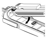
3. Rotate the battery toward the radio, and squeeze the battery and radio together until the battery "clicks" in place.
